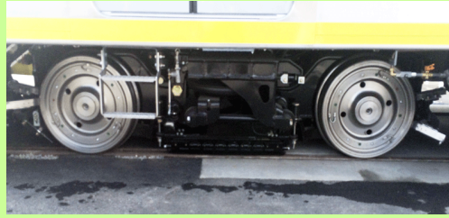
Above left: KinkiSharyo Car 1003 showing front end and coupler. Above right: Car 1003 truck with segmented track brake!
